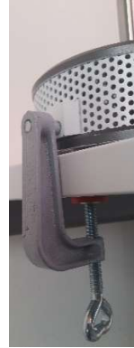
Figure 2 Secure fixing of the lamp unit with bar clamp
